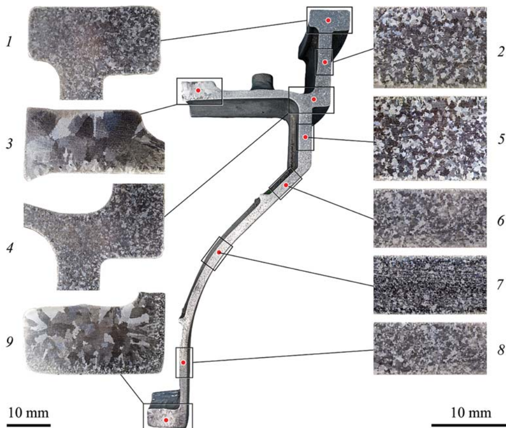
Fig. 2. Grain structure of the test casting wall (etched)
