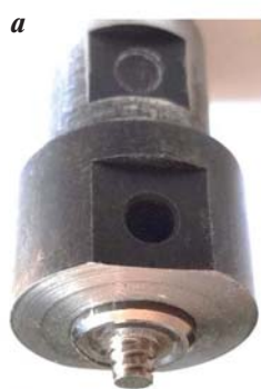
Fig. 7. Heat-resistant stir tool ( a ) and schematic drawing of multi-pass FSLW ( b )
