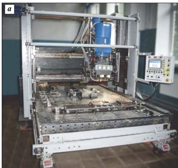
Fig. 6. FSW machine: general view ( a ) and equipment for securing restorable plate and filler material on the welding table ( b )
