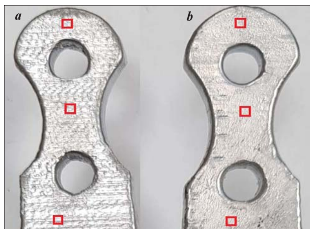
Fig. 5. External view of casting produced using non-processed model ( a ) and after its holding in dichloromethane ( b )
