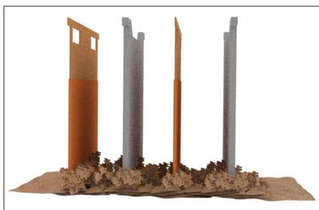
Fig. 2. Model of complete short-circuiting of the electrodes when the sludge touches the lower part of the electrodes
