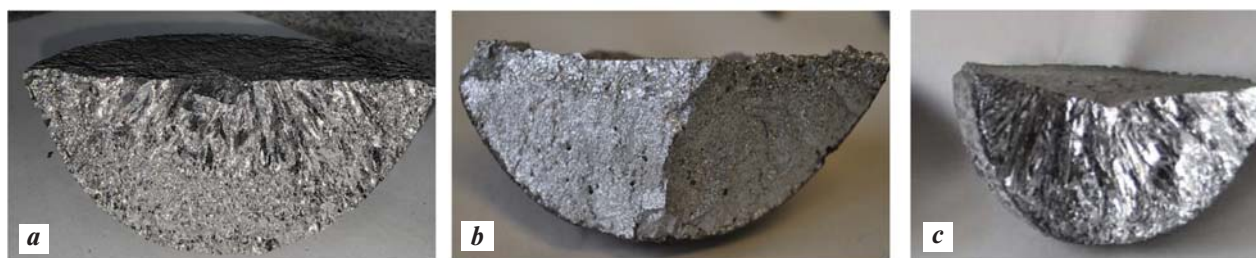
Fig. 6. External view of the macrostructure of ingots (mass 1–1.45 kg) synthesized for the Cr–Mo (Al) ( a ), Cr–W (Al) ( b ), and Cr–Al ( c ) alloys
