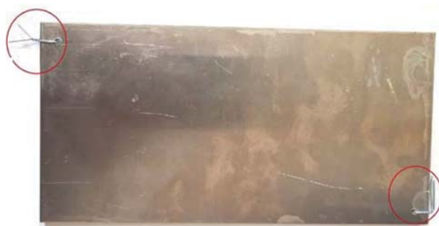
Fig. 2. Workpieces prepared for asymmetric accumulative roll bonding with preliminary joining using thin wire
