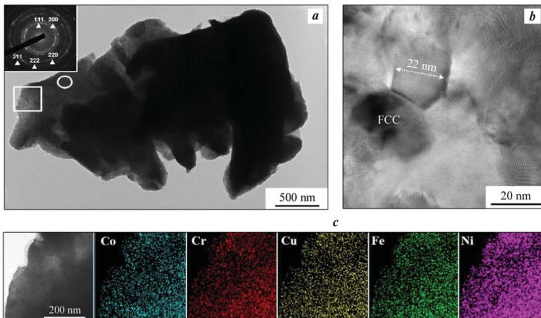
**Fig. 3.** Visualization of a CoCrCuFeNi<sub>2</sub> powder particle after 30 minutes PBM treatment (a); area within the white circle indicating the grain microstructure examination zone (b); white rectangle delineating the region analyzed via EDS (c)
