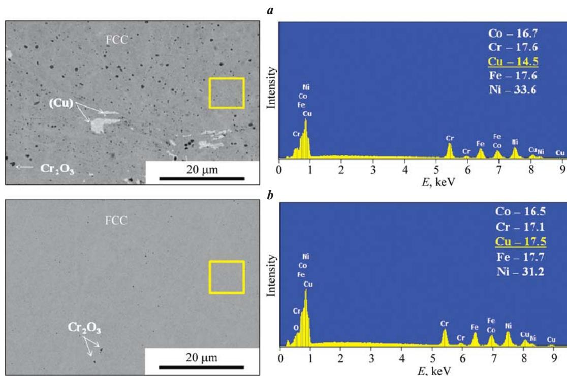
**Fig. 7.** Microstructures of CoCrCuFeNi<sub>2</sub> HEA after HP (*a*) and after HP + HT (*b*), including characteristic X-ray spectra from designated areas
