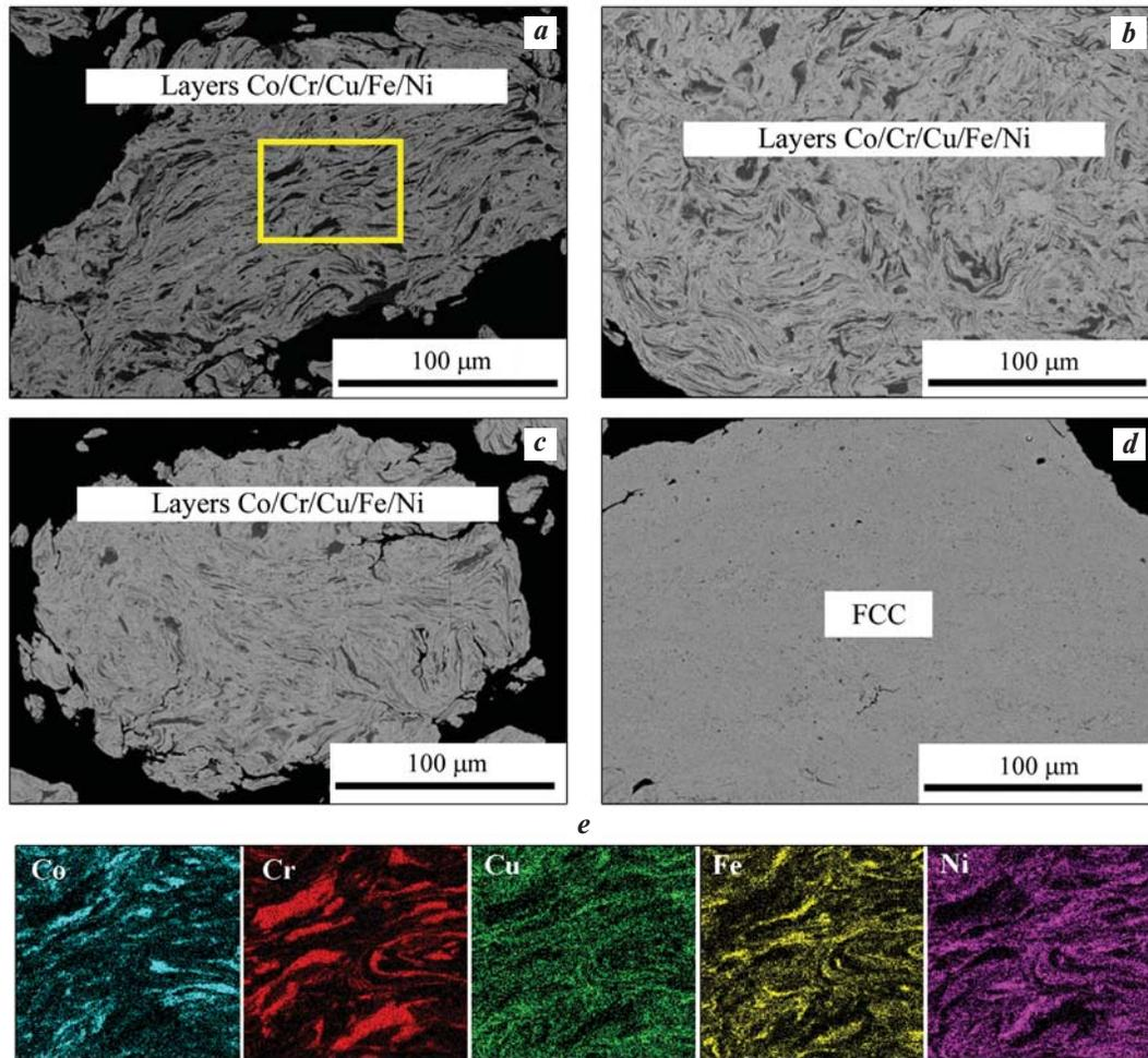
**Fig. 2.** Microstructures of  $\text{CoCrCuFeNi}_2$  powder mixtures after PBM treatment at varied durations (*a–d*) and elemental distribution maps (*e*) derived from a particle treated for 5 min, corresponding to the region indicated in image *a*
