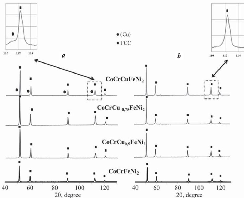
**Fig. 4.** XRD patterns of CoCrCu<sub>x</sub>FeNi<sub>2</sub> HEAs after HP (a) and HP + HT (b)
