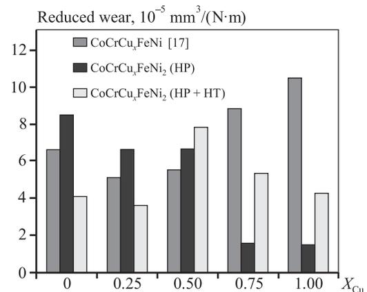
**Fig. 10.** Relationship between copper content and reduced wear rate in CoCrCu<sub>x</sub>FeNi<sub>y</sub> HEAs
