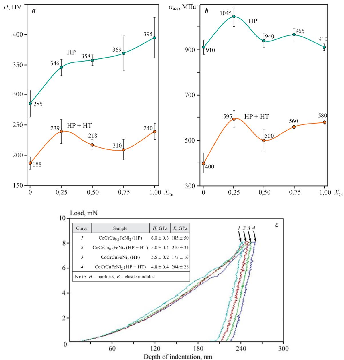
**Fig. 8.** Hardness (a), tensile strength (b) and measuring indentation (c) of CoCrCu<sub>x</sub>FeNi<sub>2</sub> HEA
