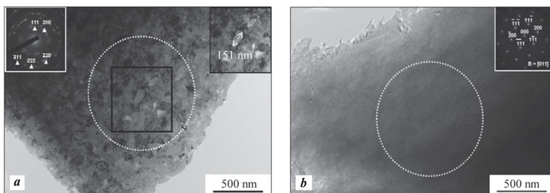
**Fig. 6.** Microstructure and electron diffraction pattern of CoCrCuFeNi<sub>2</sub> alloy samples after HP (*a*) and HP + HT (*b*)
