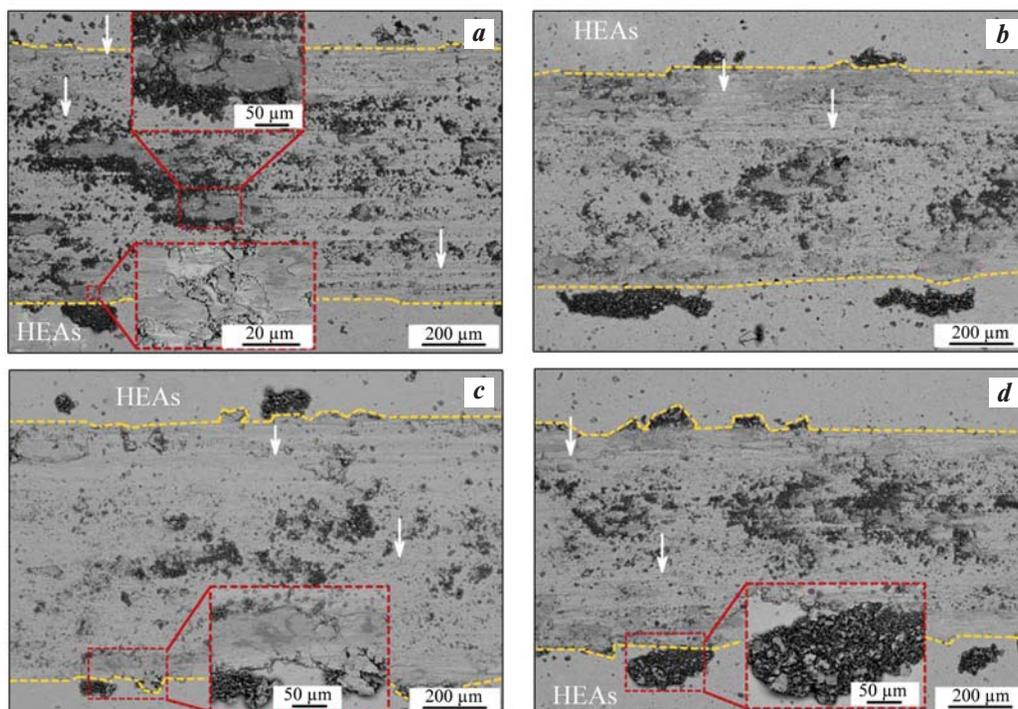
**Fig. 11.** SEM images of wear tracks on CoCrCu<sub>x</sub>FeNi<sub>y</sub> HEAs
