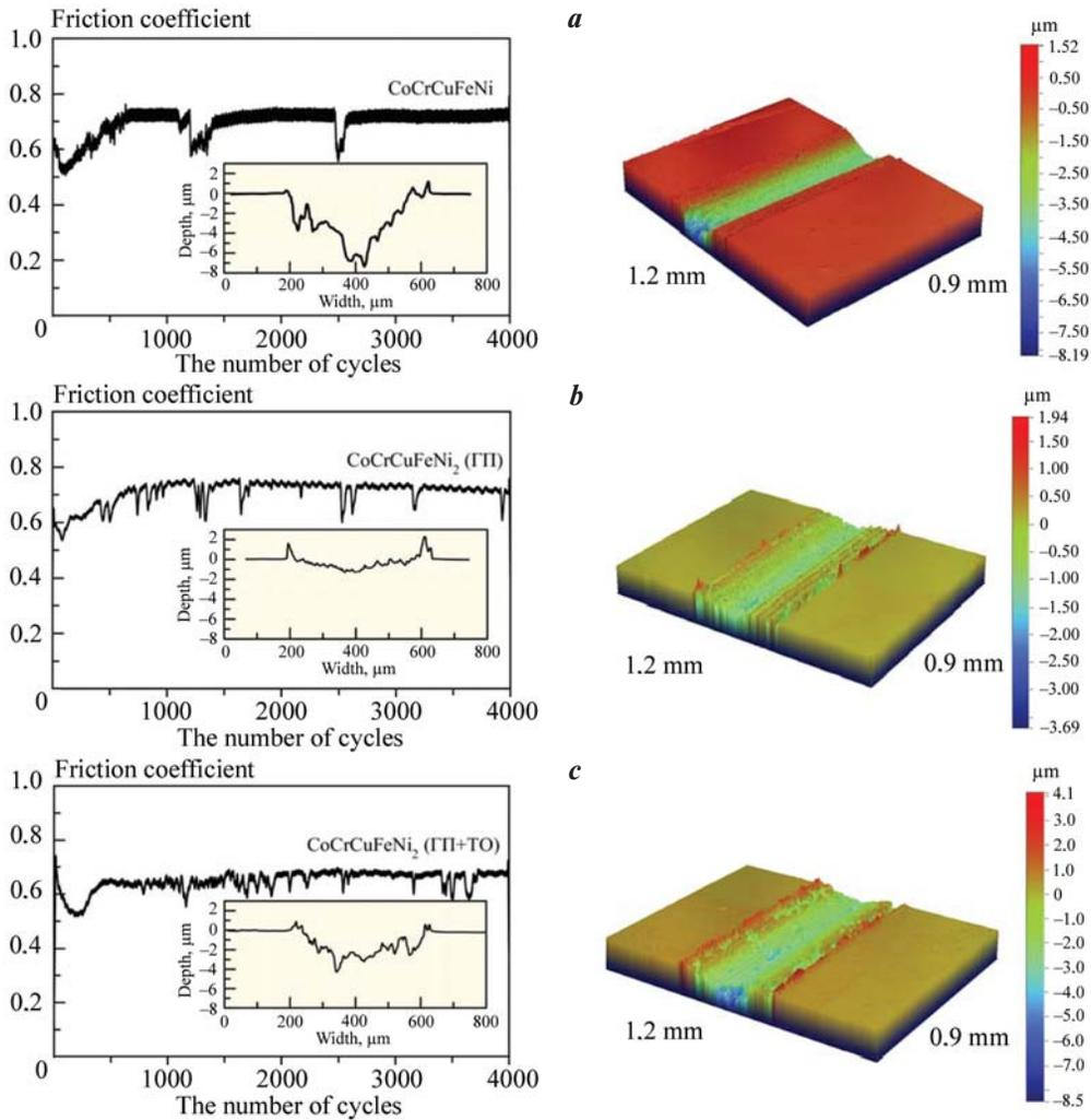
**Fig. 9.** Friction coefficient over cycle number with 3D and 2D representations of wear tracks in CoCrCuFeNi<sub>y</sub> HEAs
