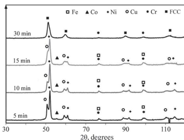
Fig. 1. XRD patterns of CoCrCuFeNi<sub>2</sub> alloy powders after PBM treatment
