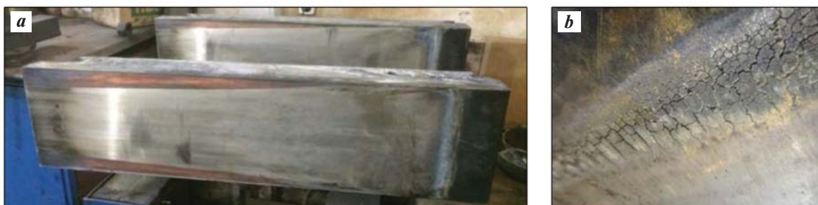
Fig. 2. Electroplated coatings defects: wear ( a ) and heat cracks ( b )
