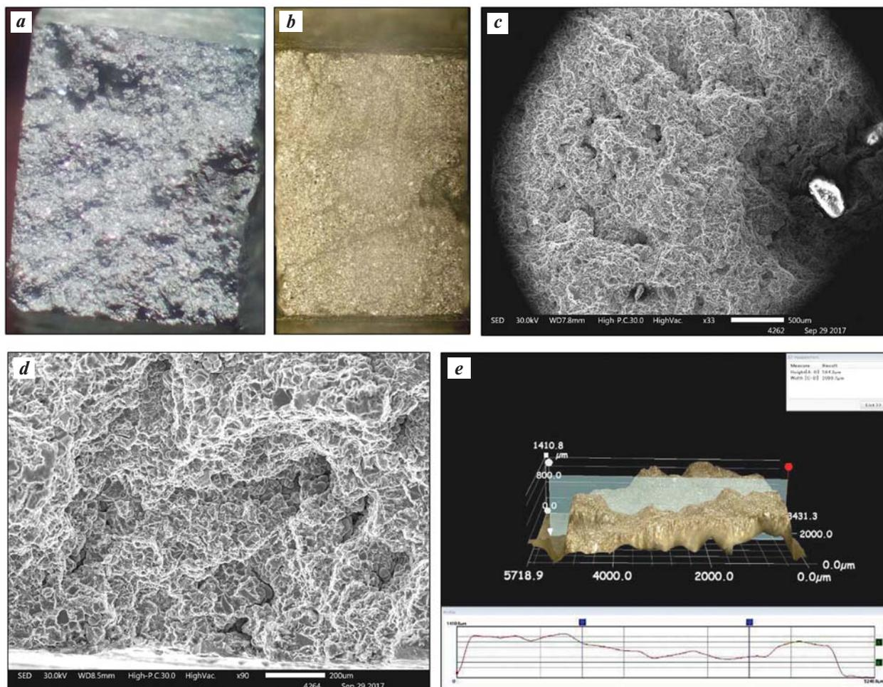
**Fig. 5.** Fracture surface of DSCM sample 1
